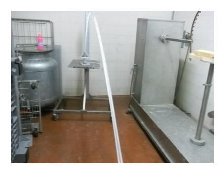
Fig. 2. - Test set-up for IPx5
