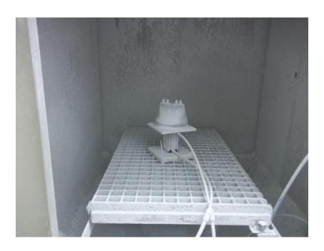
Fig. 1. - Test set-up for IP6x
