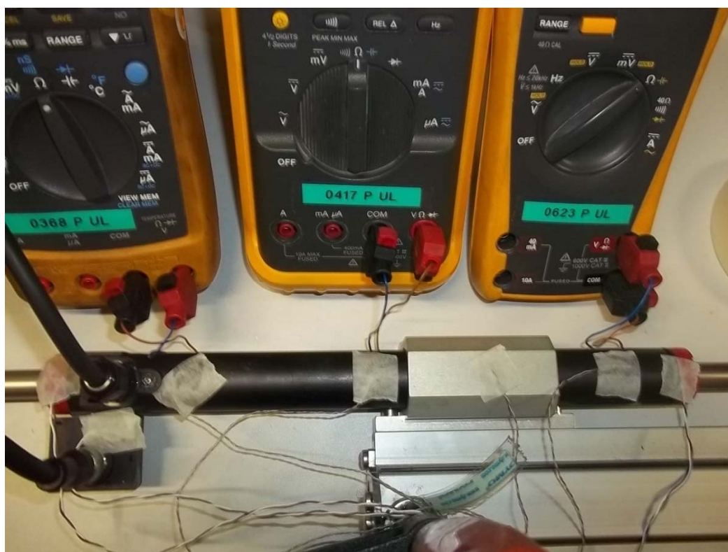
Fig. 4. - Test set-up for temperature rise test
