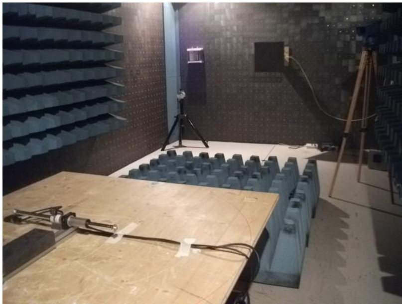
Photo test set-up for frequency above 1 GHz
