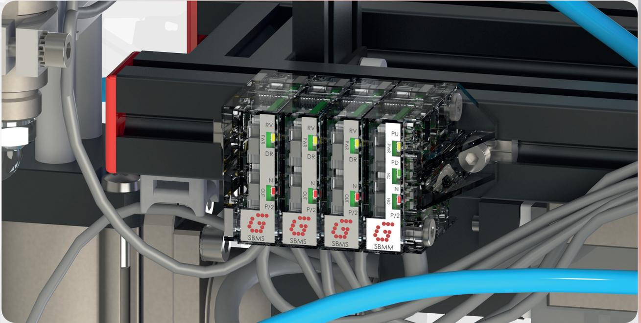
An innovative way to consider the EOAT sensor boxes. The modular sensor box SBM will allow to connect in series from 2 to 20 switches in any configuration (PNP/NPN, NA/NC), getting a single signal to allow EOAT operations.
