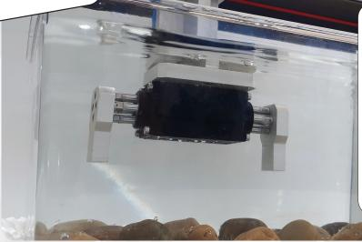
A parallel gripper, specifically designed to provide the better performances in harsh environments, internally sealed to preserve from dust, oil and also one meter underwater with protection class IP67.
